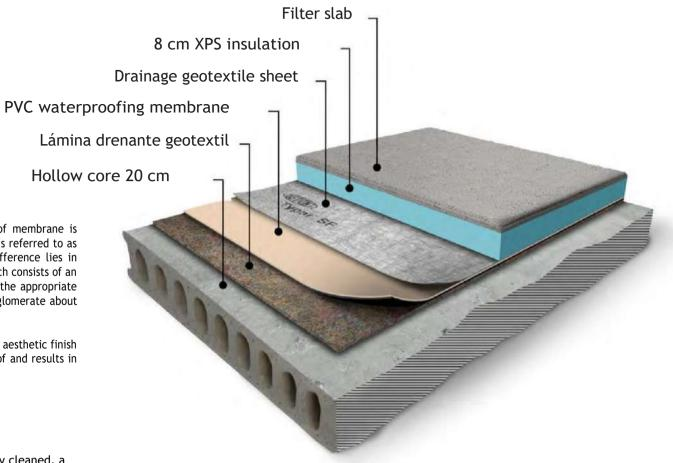
The inverted roof is called so because the waterproof membrane is placed beneath the thermal insulation. In this case, it is referred to as Inverted LF in reference to its surface finish. The difference lies in placing a filter slab on top of the waterproof layer, which consists of an insulating core made of extruded polystyrene (XPS) at the appropriate thickness, and on top of this, a layer of aggregate conglomerate about 3.5 cm thick, all in a single body.
