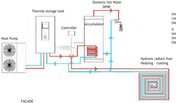
Underfloor heating is based on a circuit of water pipes that runs through the floor of the home and is capable of heating the house at low temperatures between 30° and 40°.
